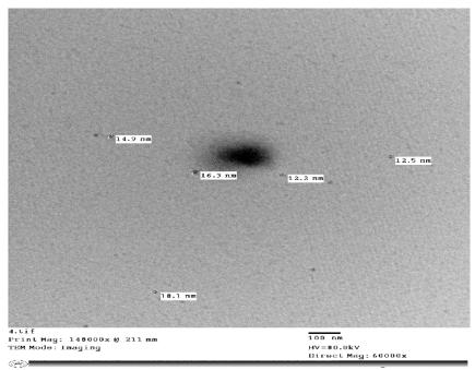
**Figure 3.** Transmission electron microscopy (TEM) image of selenium nanoparticles (Se-NPs) *synthesis* by *Bacillus subtillis*
