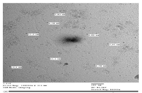
Figure 5. Transmission electron microscopy (TEM) image of selenium nanoparticles (Se-NPs) synthesis by *Streptomyces griseus*
