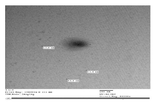
**Figure 6.** Transmission electron microscopy (TEM) image of selenium nanoparticles (Se-NPs) synthesis by *Trichoderma harzianum*
