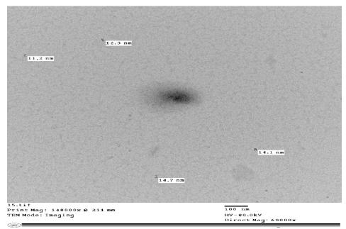
**Figure 7.** Transmission electron microscopy (TEM) image of selenium nanoparticles (Se-NPs) synthesis by *Chaetomium globosum*
